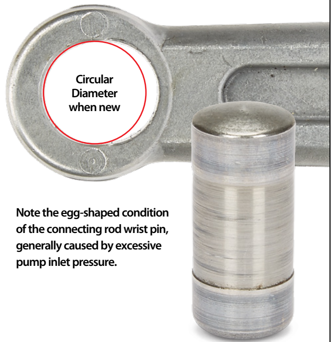
Connecting Rod and Pin
